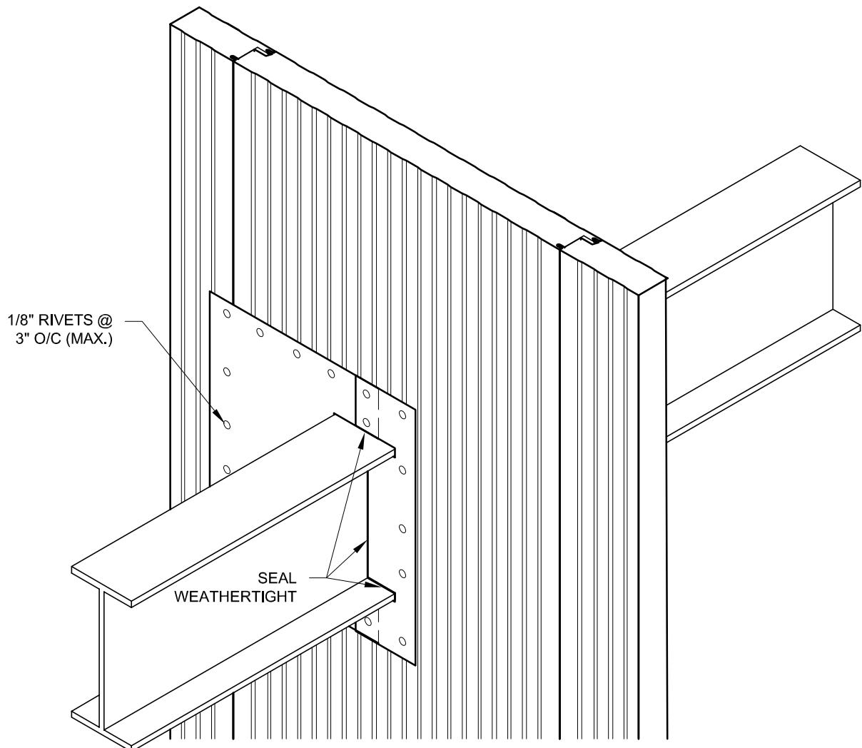
PENETRATIONS THROUGH INSULATED PANELS - FINAL ASSEMBLY
