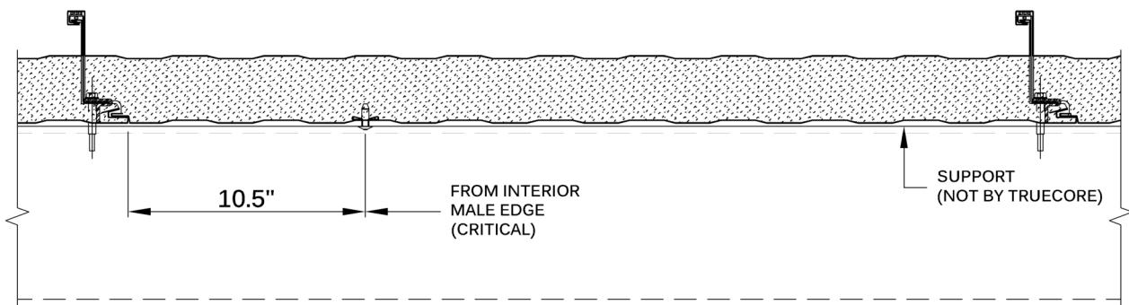
(FP2) SIDE JOINT AND (1) BULB-TITE® RIVET
