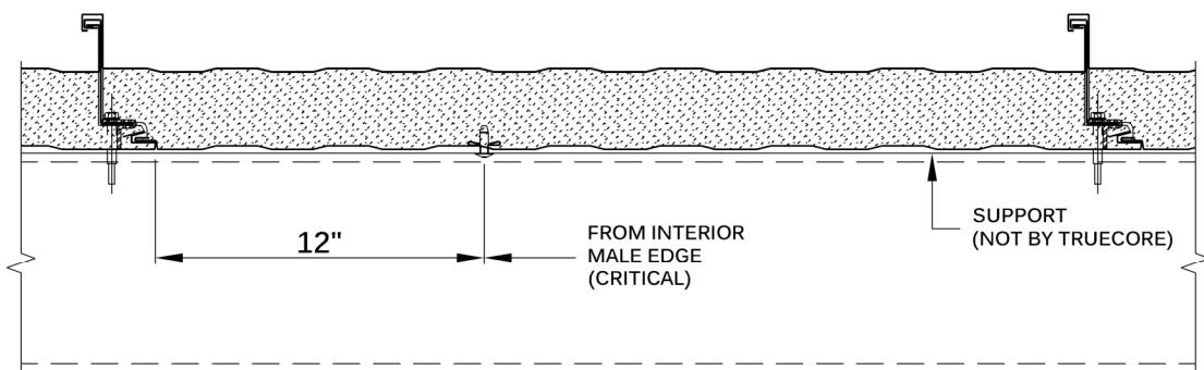
(FP2) SIDE JOINT AND (1) BULB-TITE® RIVET
