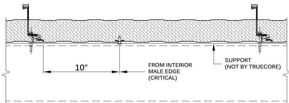
(FP2) SIDE JOINT AND (1) BULB-TITE® RIVET
